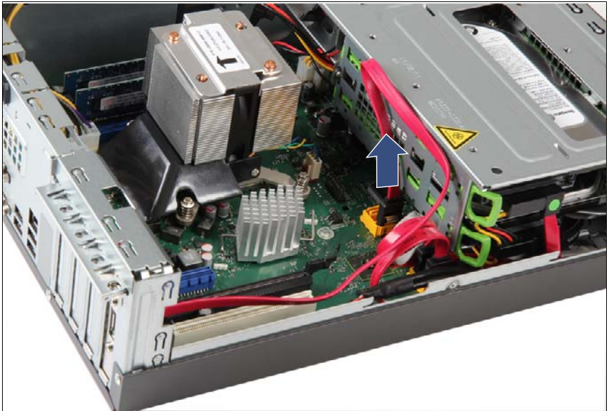
Figure 105: Disconnecting the eSATA cable
